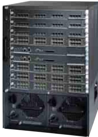
The Cisco MDS 9509 for IBM System Storage offers 1, 2, 4, 8 and 10 Gbps link speeds with up to 336 Fibre Channel ports in a 14U enclosure
